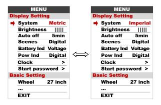
**8.2 Brightness**: Press Up / Down button to change the brightness of the backlight, I is darkness, IIIII is brightness
