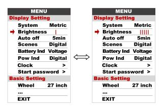
**8.3 Auto off :** Press UP/DOWN button to change the auto power off time, from 1 to 9, the number represent time (minutes) to shutdown, default value is 5 minutes.
