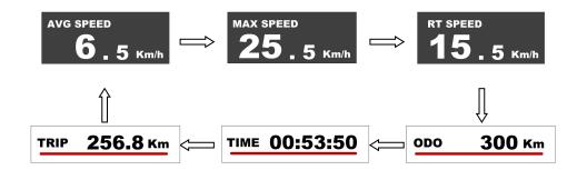
\*\*If there is no operation for 5 seconds, display will return Speed (Real-Time) display automatically.
